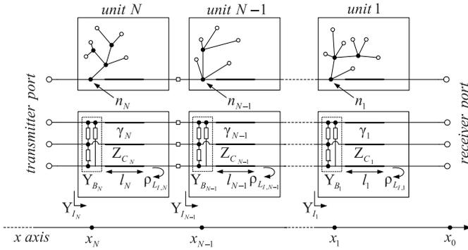
Fig. 2. On the top, unifilar description of the remapped topology. On the bottom, the correspondent representation in units.
