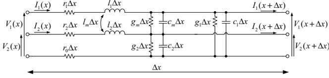
Fig. 1. Equivalent per-unit-length representation of a section of three conductors line.
