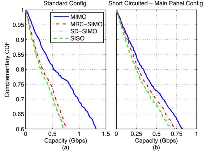
Fig. 3. Complementary cumulative distribution function of the capacity for different schemes in (a) the standard networks, (b) the SC-MP networks.
